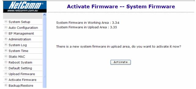
If you don't upload 'System Firmware' first, the 'Upload Area' is blank,
